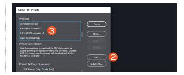
The installation is successful when the "K-Print PSO coated v3" becomes visible in the list of "presets".
